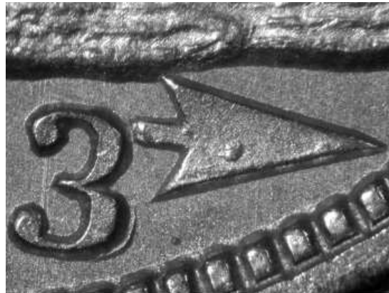
Die defect on right arrow
