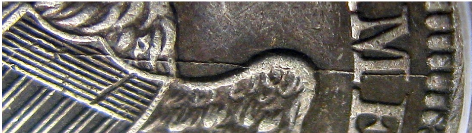
Die Crack #2 (above)
