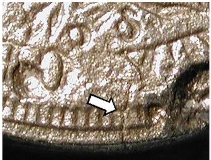
Perfect match of die crack and mintmark on coin and the die
