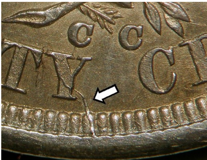
Perfect match of die crack and mintmark on coin and the die
